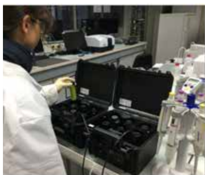
Left: ALERT LAB being used in a water quality analysis laboratory. Middle: The equipment during a field operation, analysing six samples simultaneously. Right: ALERT LAB as used by regulatory agency agent in the field.
